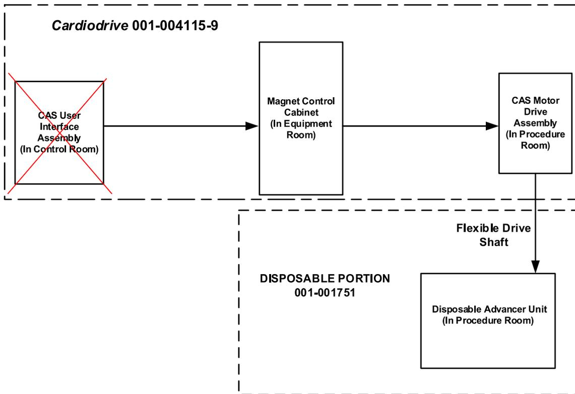
**Figure 2.** *Cardiodrive* interconnect diagram
